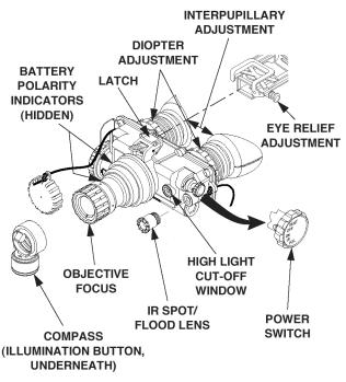
NOTE - LOW BATTERY INDICATOR AND IR SOURCE "ON" INDICATOR ARE VISIBLE IN RIGHT AND LEFT EYEPIECE LENSES, RESPECTIVELY.
